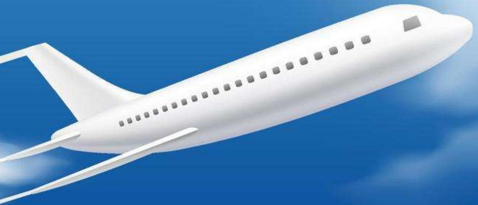
Engineers try to make drag as small as possible by giving aeroplanes a smooth shape, but they still gobble up huge amounts of fuel to keep flying fast enough to generate lift.
