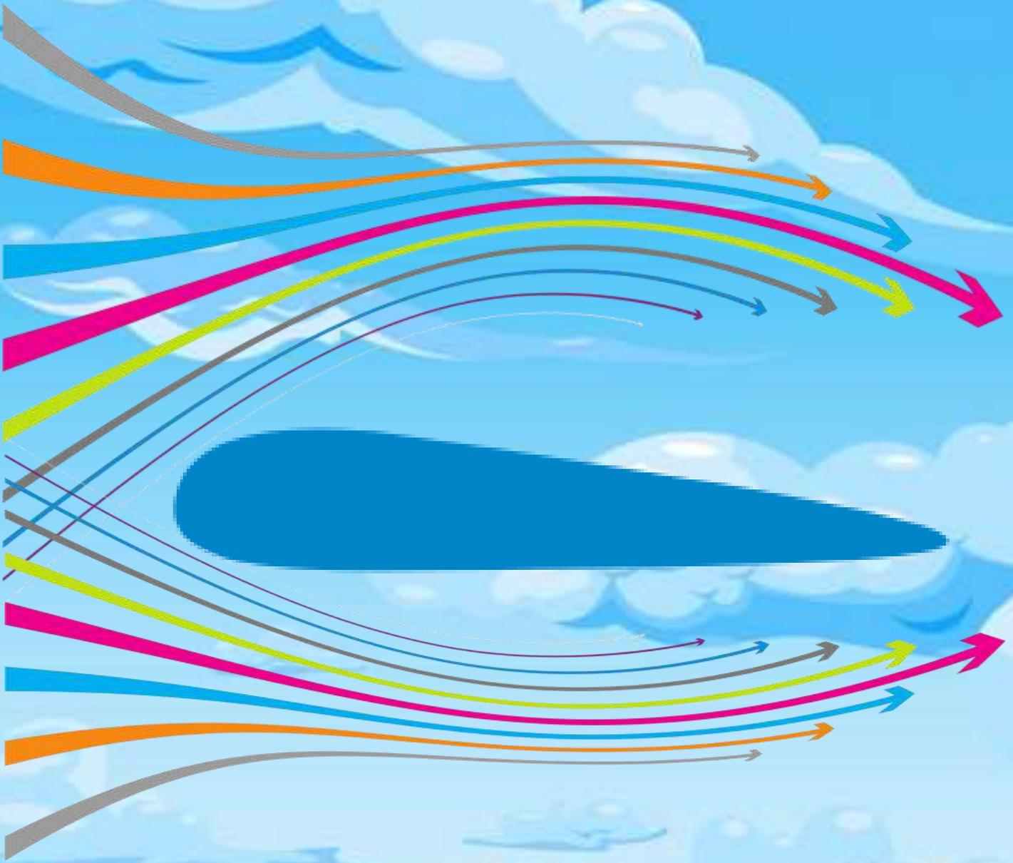
Each idea is good, but neither can completely explain lift on its own. The answer is probably a mixture of all these things: the downwards flow of air, the speed of air above the wing, AND the difference in pressure.
